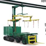
terrains and increased slopes, the upper assembly will automatically level itself for increased stability and ease of panel placement.
