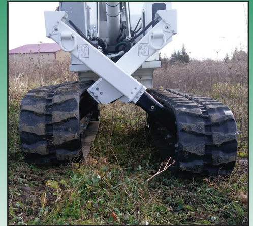
Independently Adjustable Tracks 8" of Vertical Slope Adjustment
